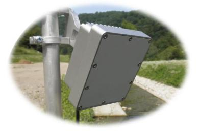
**RV7** is a non-contact 24.125/24.200 GHz RADAR based velocity sensor that uses Doppler Effect to produce velocity data of a moving surface. The measurement can be widely used for hydrological monitoring, flood control, and environmental pollution monitoring. Non-contact surface flow measurement is simple, free from water corrosion, silt or slurry. It also protects the safety of personnel.
